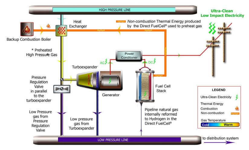
\* Pre-heating is required because gas cools as its pressure is reduced. The Direct FuelCell<sup>®</sup> provides thermal energy for pre-heating and therefore the boiler is only required for backup.
